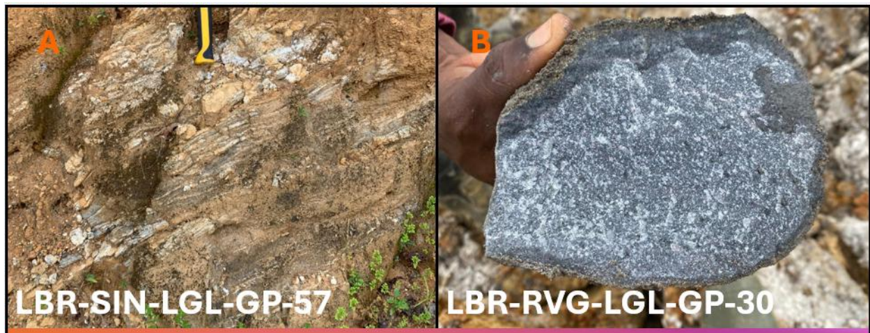
A – A highly weathered granitic gneiss exposed along road cut enroute to Nyennawilken ASM field B – A sample of ultramafic (diabase) taken from an active ASM pit in “Somalia”
